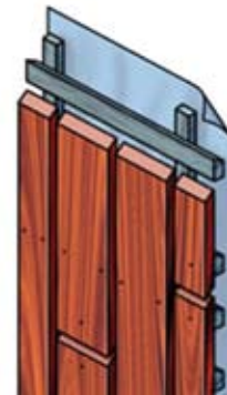
Verticale open gevelbekleding.
